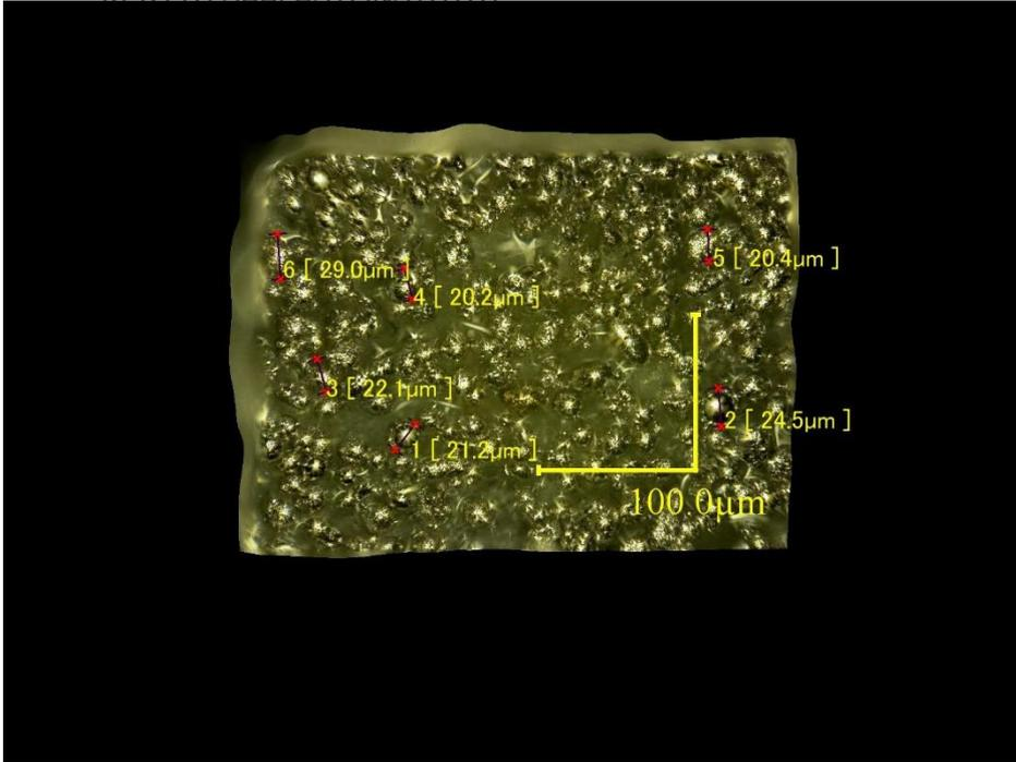
**Fig.4** powder particles in microscopic image
