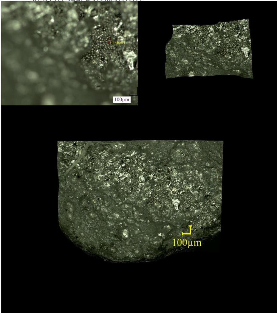
**Fig. 3** Microscopic image of the tensile test bar (upper left closer image in fracture plane, upper right is 3D image in fracture plane and lowest is bigger area image)
