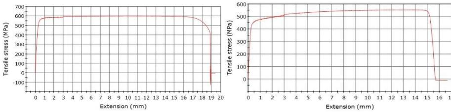
**Fig. 2** Tensile tests for AISI 316L (without heat treatments on the left and heat treated on the right side)
