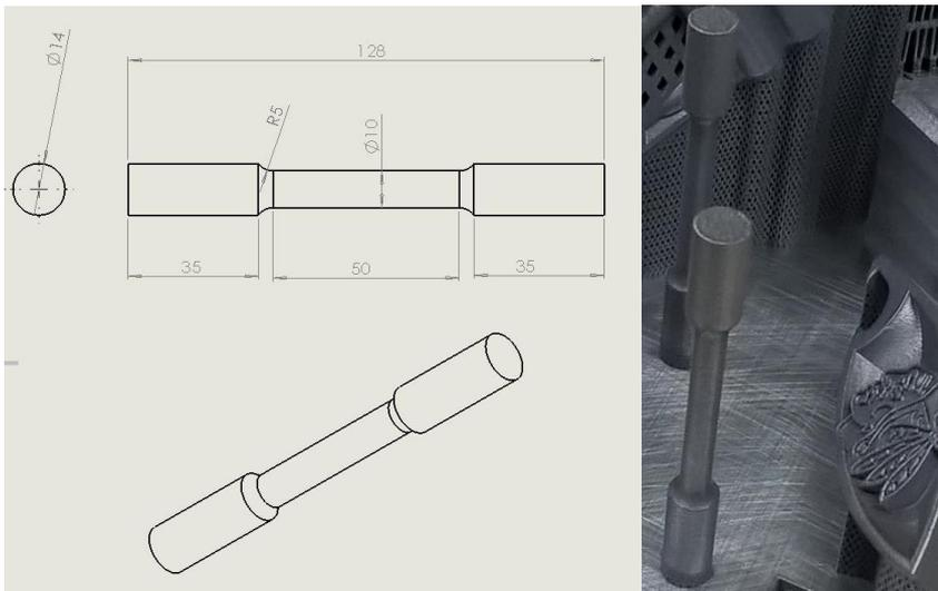
**Fig.1** Tensile test bar and 3D-printing orientation
